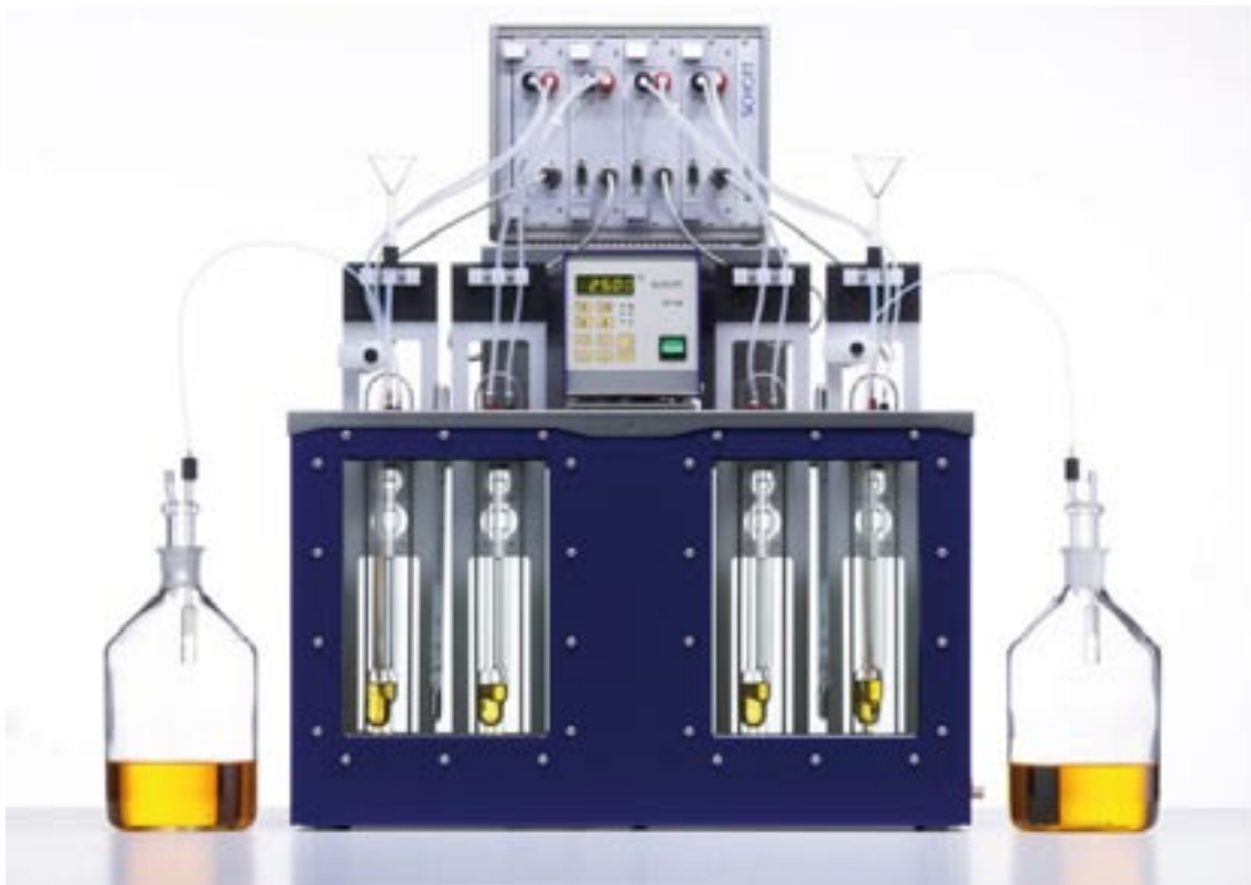
Analytical testing equipment for the determination of the IV of PET - Schott, Mainz
