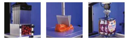
The TA1 texture analyser is a cost effective, easy to use solution for performing rapid, detailed texture analysis tests on applications up to 1 kN (225 lbf).
