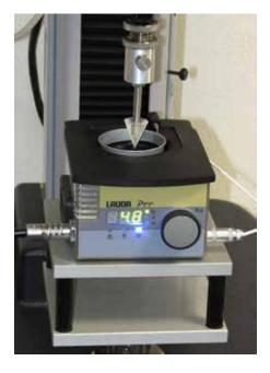
Penetration test with peltier system able to generate temperature from 5°C to 80°C.
